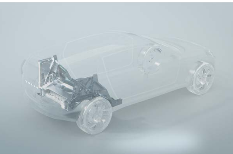
The megacasting cell manufactures the vehicle's rear underbody as a single aluminium part, replacing about 100 conventionally manufactured and assembled components
