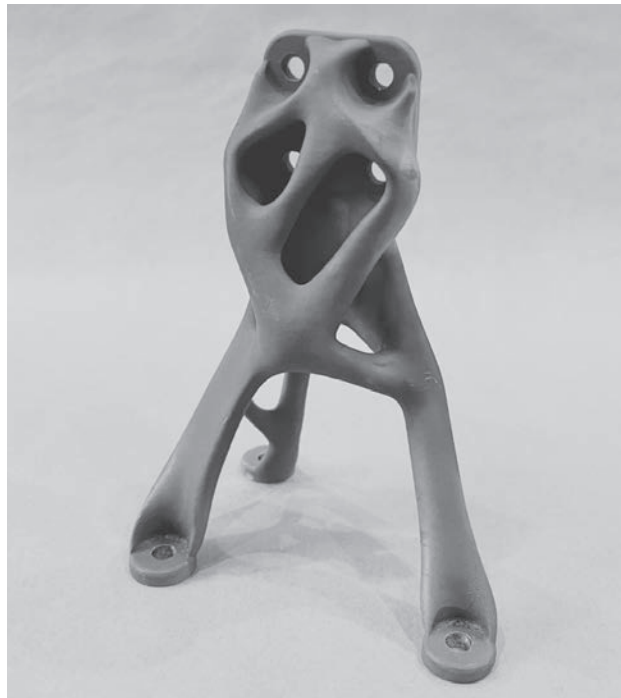
An A15 bracket developed by NASA as part of the Text-to-Spaceship and Evolved Structures research, cast by Fabri. CAD to casting in 5 days. Winner of the 2026 AFS Casting of the Year (Small Foundry)
